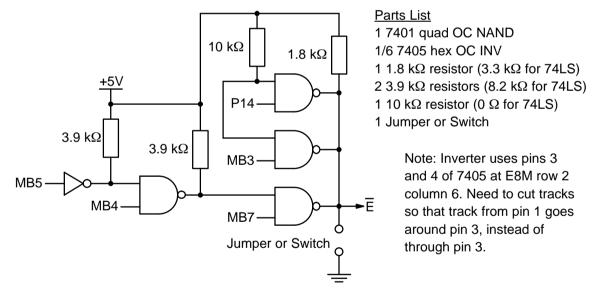
This design only requires one additional 7401 quad open collector NAND and four resistors. An additional inverter is a spare from the existing design. With the jumper or switch in the on position, the original EDUC–8 instruction set is used.
