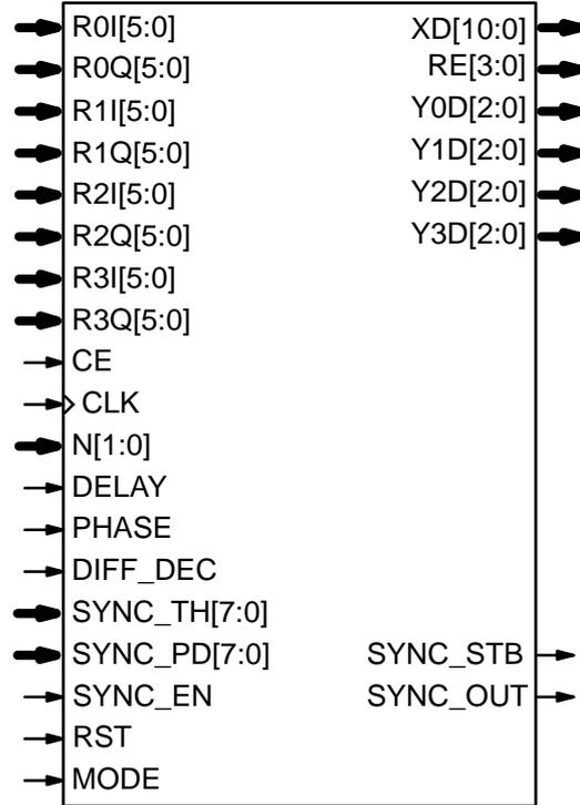
Figure 1: VA06C schematic symbol.
