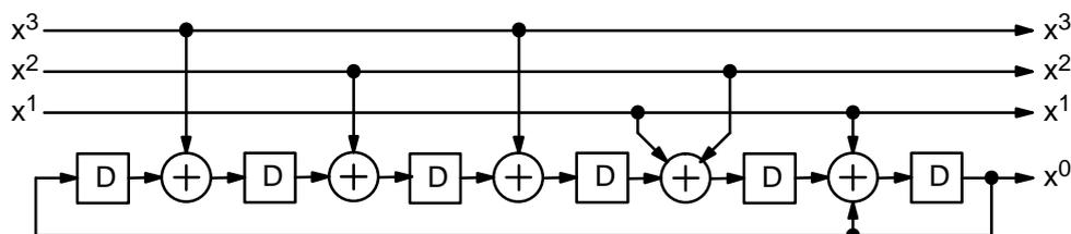
Figure 2: 64 state rate 3/4 systematic convolutional encoder.
